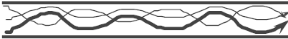
fiber optic multi-mode graded-index
