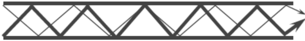
fiber optic multi-mode step-index
