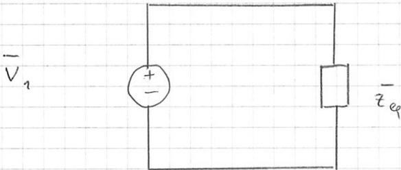
$$\bar{z}_{eq} = \frac{\bar{z}_1 \cdot \bar{z}_2}{\bar{z}_1 + \bar{z}_2} = 10,22 \cdot e^{j42,36^\circ}$$
