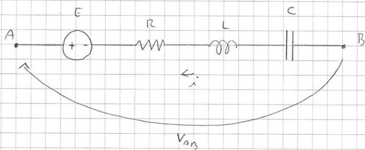
$$V_{AB}(t) = E(t) - L \frac{di(t)}{dt} - Ri(t) - \frac{1}{C} \int i dt$$
