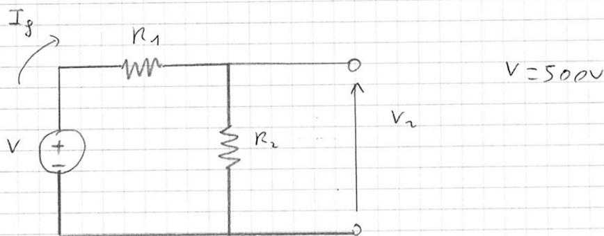
$$\left. \begin{array}{l} R_1 = ? \\ R_2 = ? \end{array} \right\} \begin{array}{l} V_2 = 50V \\ I_g = 10mA \end{array}$$
