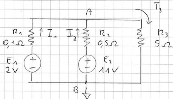
$$V_B = 0 \text{ V} \Rightarrow V_A = V_{AB}$$
