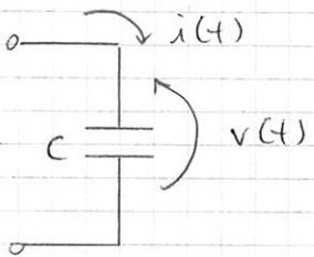
$$v(t) = \frac{1}{C} \int i(t) dt \rightarrow \bar{V} = \frac{1}{j\omega C} \bar{I} = -j \frac{1}{\omega C} \bar{I}$$
