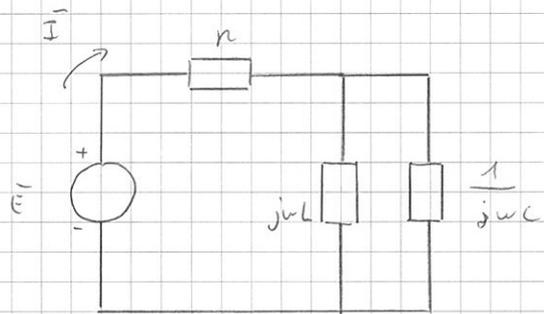
$$\bar{z} = R + \frac{1}{\frac{1}{j\omega L} + j\omega C} = R + \frac{j\omega L}{1 - \omega^2 LC}$$
