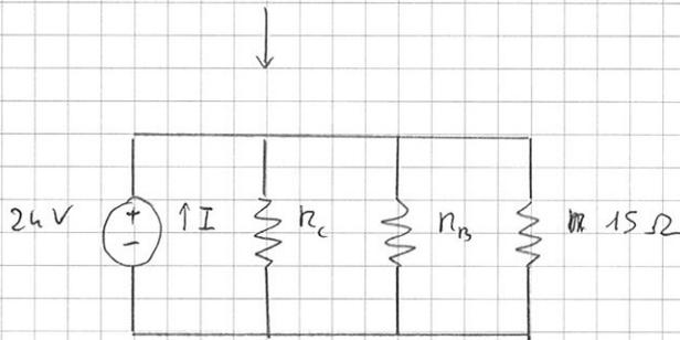
$$I = \frac{24}{R_B \parallel r_c \parallel 15 \Omega} = \frac{24}{1} = 4,27 \text{ A}$$
