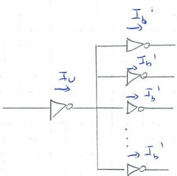
$$\left\{ \begin{array}{l} V_{CC} - n_c I_u = V_u \\ I_u = \frac{V_u - V_f}{n_B} \quad m = m I_b' \end{array} \right.$$
