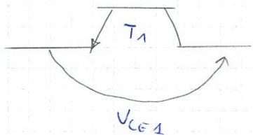
$$V_{CE1} = V_f - V_i \underset{t > 0}{\underset{\parallel}{\parallel}} V_f - V_{CESAT} > V_{CESAT}$$
