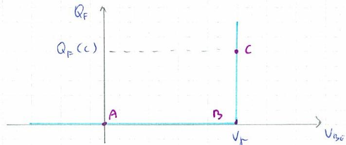
$$* \frac{V_{CC} - V_F}{R_B} = \frac{Q_F}{\beta_F \tau_F} + \frac{dQ_F}{dt}$$
