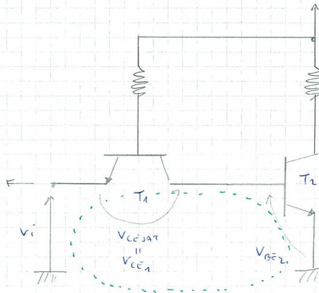
$$V_{BE2} = V_i + V_{CE} = V_{CE,SAT} + V_{CE,SAT} < V_f$$
